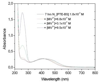
Figure 7. Evolution of the absorption spectra for PTE-BS as a function of the concentration of the quencher added.
