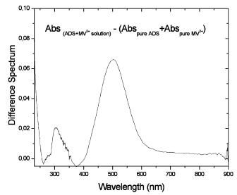
Figure 9. Difference spectrum obtained by subtracting from the absorption spectrum of a solution of PTE-BS and MV<sup>2</sup>the addition of the absorption spectra of the pure substances.
