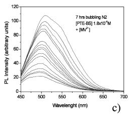
**Figure 5.** Fluorescence spectra of water solutions of PTE–BS (excited at 400 nm) in the presence of MV<sup>2+</sup> for concentrations of PTE–BS: (a)  $1.8 \times 10^{-4}$  M with nitrogen bubbling for 7 h, (b)  $9.0 \times 10^{-4}$  M with oxygen, and (c)  $1.8 \times 10^{-4}$  M with oxygen.
