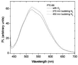
Figure 2. Fluorescence spectra (excited at 400 nm) of PTE- $BS(8 \times 10^{-5} \text{ M})$  aqueous solutions taken during the getting rid off oxygen process.
