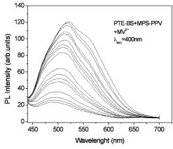
**Figure 12.** Fluorescence spectra of an aqueous mixture (50/50 v/v) of PTE-BS  $(1.8 \times 10^{-4} \text{ M})$  and MPS-PPV  $(1.8 \times 10^{-4} \text{ M})$  excited at 400 nm, in the presence of MV<sup>2+</sup>.
