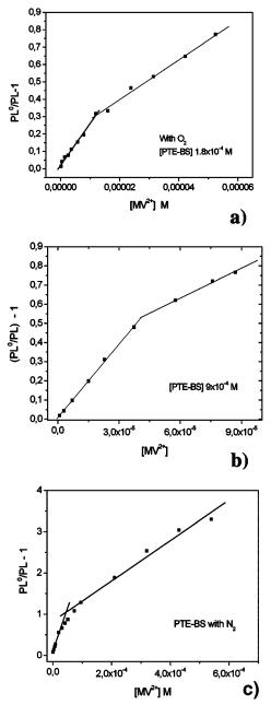
Figure 6. Stern-Volmer plot for quenching of the fluorescence by MV<sup>2+</sup> for PTE-BS aqueous solution of concentrations: (a)  $1.8 \times 10^{-4}$  M with nitrogen, (b)  $9.0 \times 10^{-4}$  M with oxygen, and (c)  $1.8 \times 10^{-4}$  M with oxygen.
