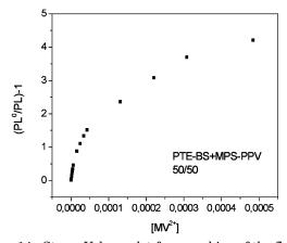
**Figure 14.** Stern-Volmer plot for quenching of the fluorescence by MV<sup>2+</sup> of the 50/50 v/v mixture (excited at 400 nm) of PTE-BS and MPS-PPV.
