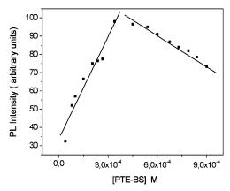
**Figure 4.** Fluorescence intensity (excited at 400 nm) as a function of the concentration of PTE-BS in aqueous solutions.
