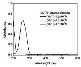
Figure 8. Evolution of the absorption spectra for pure MV<sup>2+</sup> as a function of the concentration.
