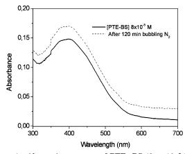
Figure 1. Absorption spectra of PTE-BS (8  $\times$  10<sup>-5</sup> M) in water with oxygen (solid line) and after 2 h of nitrogen bubbling through the solution.
