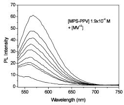
**Figure 10.** Fluorescence spectra of a water solution of MPS-PPV (excited at 500 nm) in the presence of  $MV^{2+}$ .
