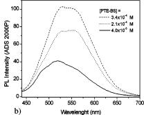
Figure 3. Fluorescence spectra (excited at 400 nm) of PTE-BS in aqueous solutions showing (a) PL increases upon dilution from  $9 \times 10^{-4}$  down to  $3.4 \times 10^{-4}$  M and (b) PL decreases upon dilution from  $3.4 \times 10^{-4}$  down to  $4.0 \times 10^{-5}$  M.
