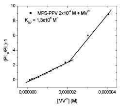
**Figure 11.** Stern–Volmer plot for quenching of the fluorescence by  $MV^{2+}$  for MPS–PPV aqueous solution of concentrations 1.9  $\times$   $10^{-4}$  M.
